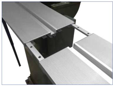
Attach the removed leg to the far end of the add-on guide and with the attachment bars secured to the first guide, slide the Add-on Guide onto the bars as shown above. Slide the track together and secure track using the set screws an a hex key wrench.
