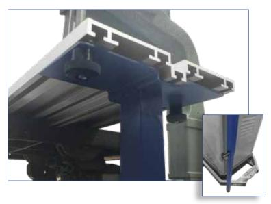
Place each leg toward the outer edge of each end of the Super Wide Miter Guide for optimum support. Secure each leg using the supplied T-bolts and Knobs as shown above. Once the legs are secure, adjust the legs and feet so that the feet sit firmly on the floor.
