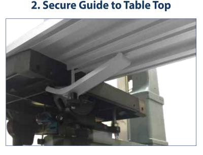
Using the two aluminum hold downs (1 on each side of the table), secure the Super Wide Miter Guide to your band saw table top as shown above.
