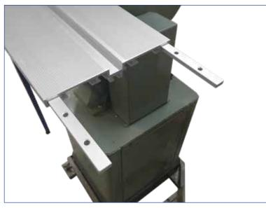
Slide the two bars into the tracks under the Super Wide Miter Guide that is on the band saw table. Leave about half of the bars out from the edge of the guide. Secure the bars using the set screws and a hex key wrench.
